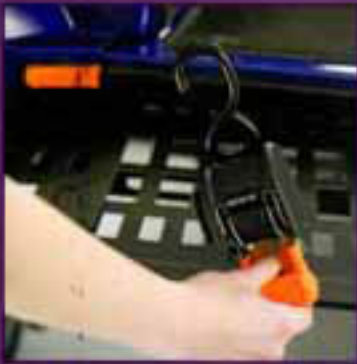
Self-Tensioning Retractable Securement Belts - One Hand Operation
